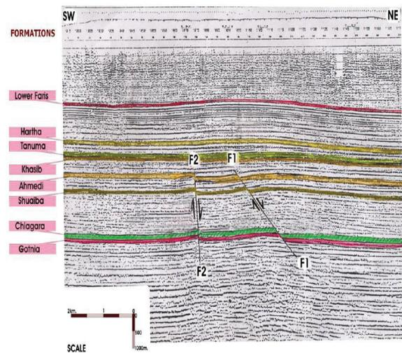
**Figure 2.** Seismic cross section with hydrocarbon source, reservoir, and seal rock units in East Baghdad Oil Field. Double line arrows indicate directions of migration pathways, while F1 and F2 are normal faults (modified after Al-Ameri, 2011).
