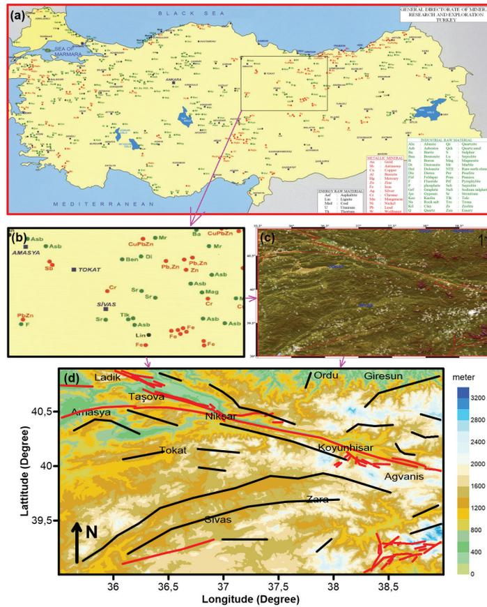
Figure 7. (a) Turkey ore deposits map (URL-2, 2020), (b) ore deposits map of study area, (c) seismicity of the region, (d) known faults have been compiled from ISC (in red) and found lineaments (in black).
