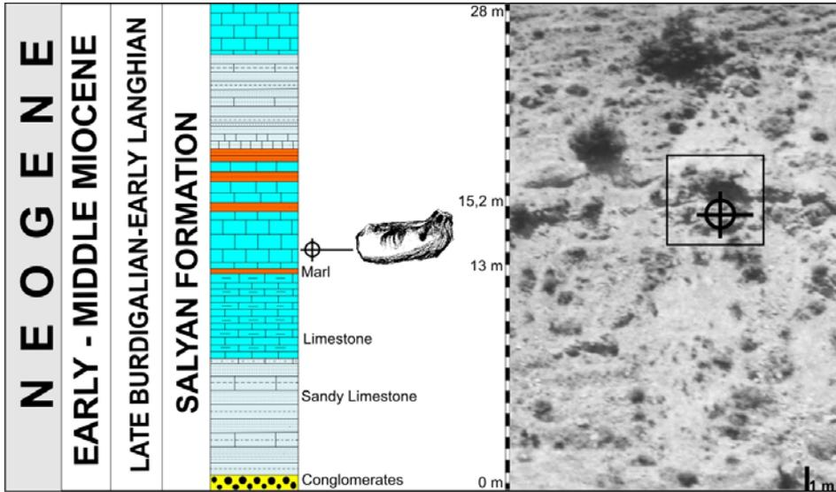
Figure 2. Measured stratigraphic section from Salyan Formation (Hoşgör, 2008).
